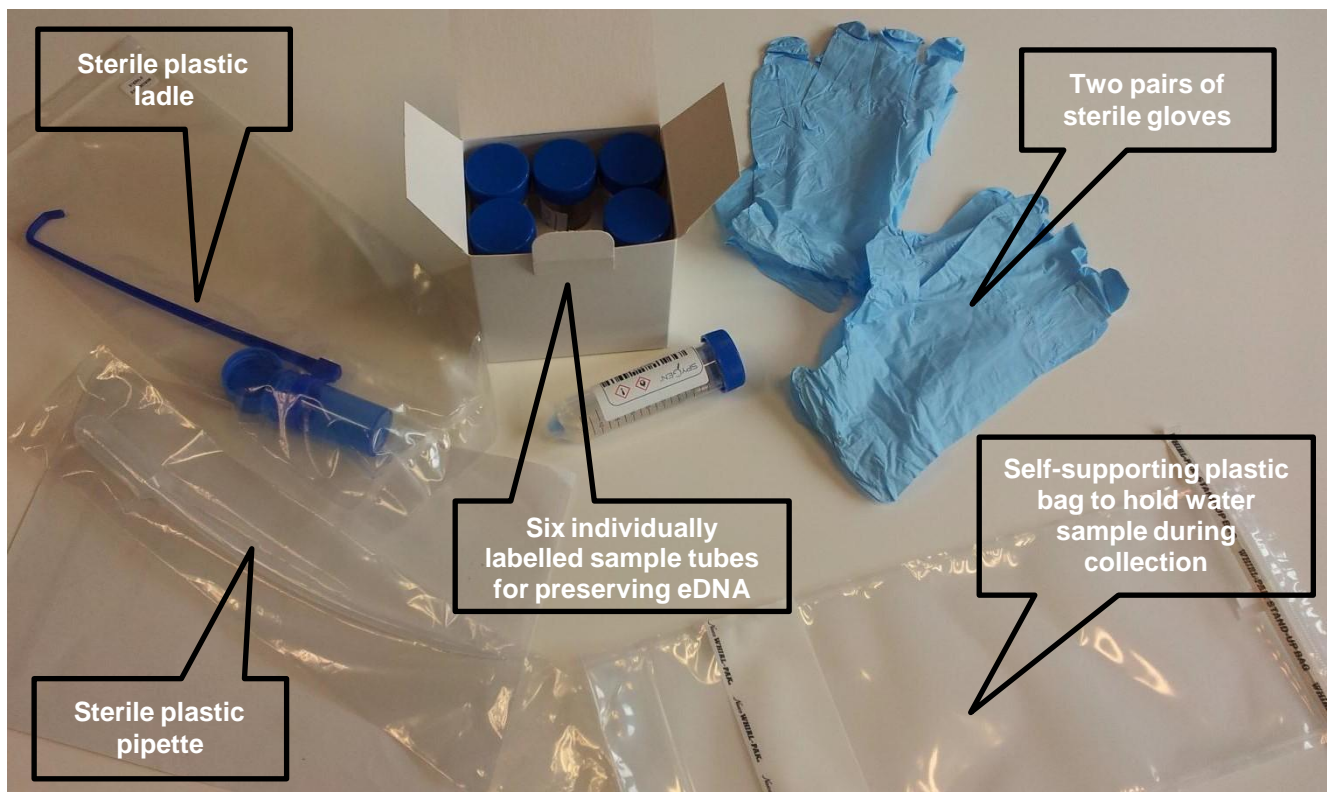
Figure 2 Sampling equipment used for eDNA water samples by Biggs et al. (2014)
