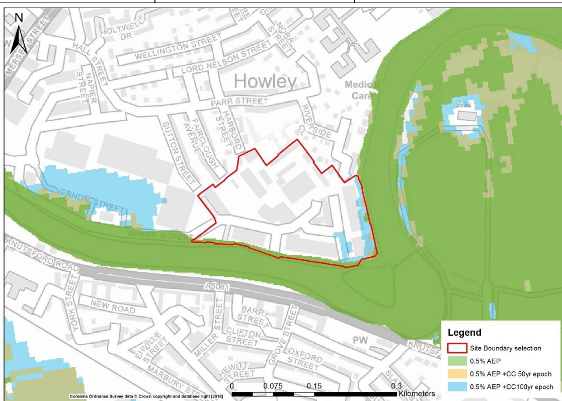
Figure 3.9.3 Defended tidal outlines for 0.5% AEP and 0.5% AEP with 50yr (2065) and 100yr (2115) climate change increases
