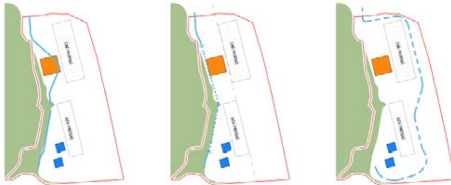
Figure 4.8: Brook diversion Options – Existing Location; Culverted; Diverted
