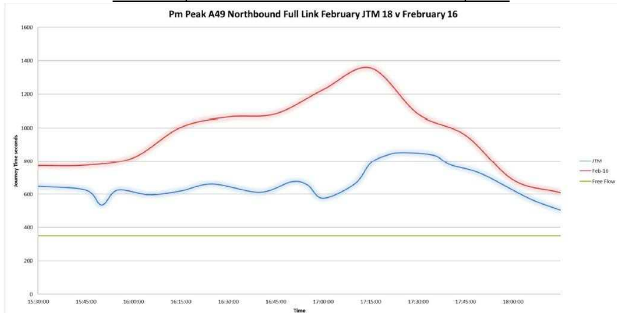
Figure 54: PM Peak A49 Northbound Journey time comparison between JTM data used from the WITS system 2018 and information from Basemap 2016
