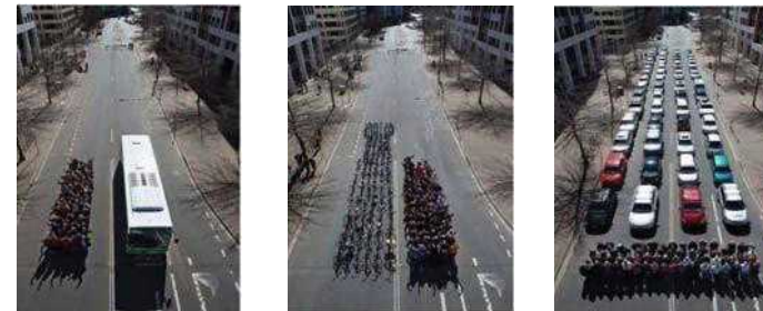
Figure 16: Difference in road space requirement for 60 pedestrians, cyclists, bus users and car drivers
