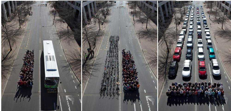
Figure 34 Use of available highways capacity for the transportation of 60 people for pedestrian, cycle, bus and car travel
