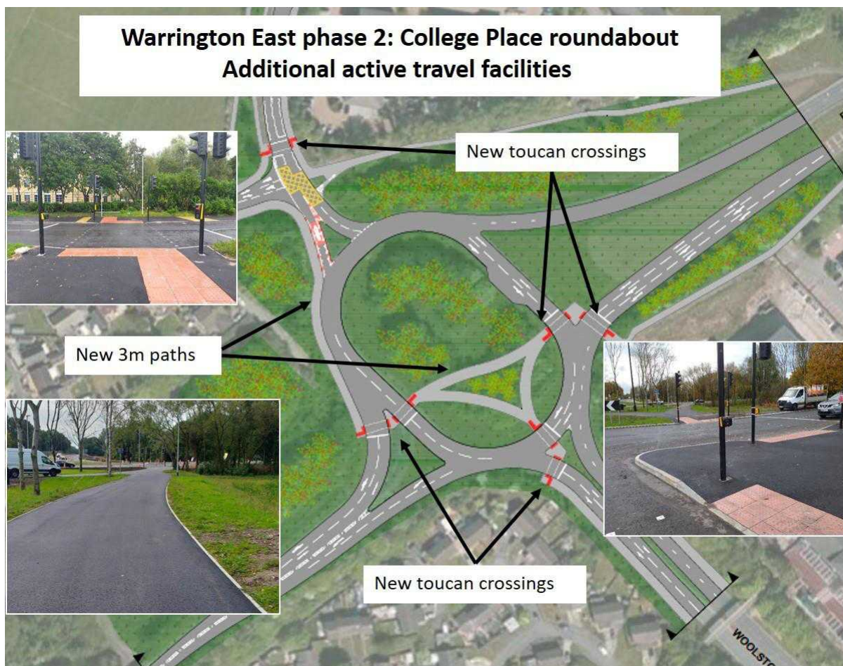
College Place roundabout – new crossings and paths
