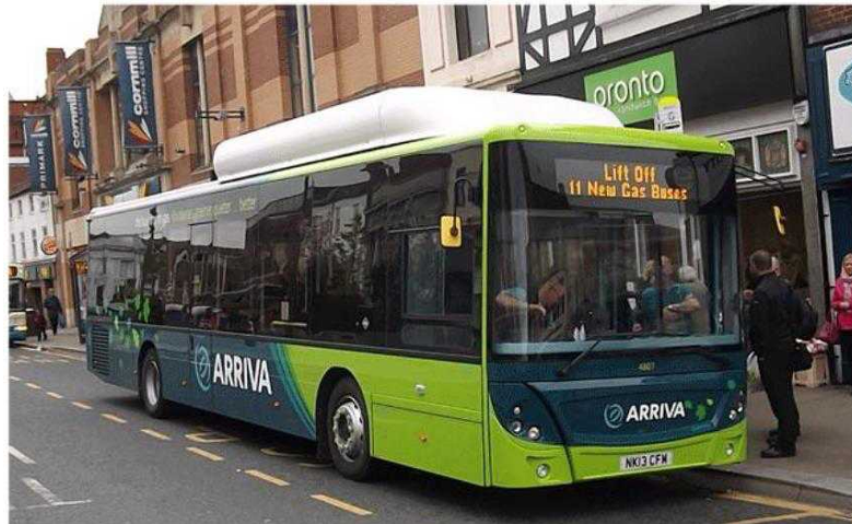
Figure 123 Arriva Hydrogen fuel cell bus - 70 passenger capacity
