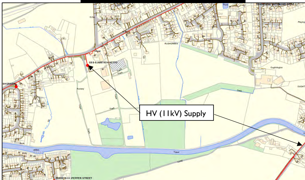
Figure 4.1 Electricity Infrastructure (SP Manweb)
