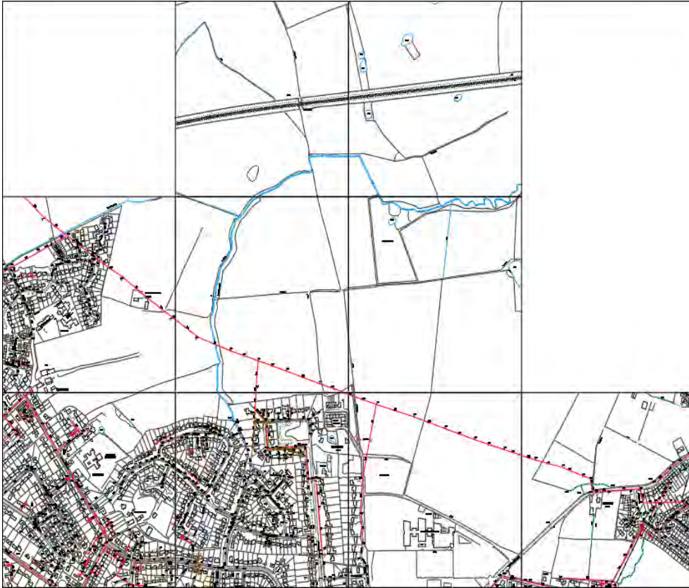
Figure 3.1 Combined UU Sewer Plan
