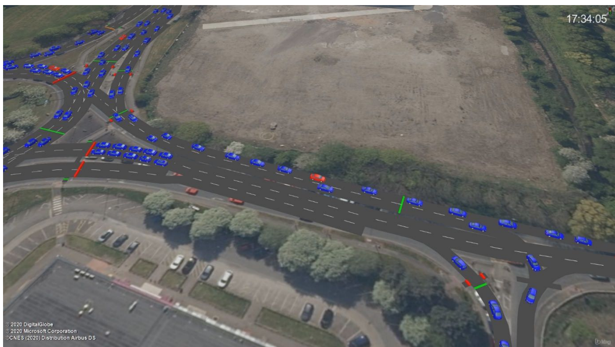
Figure 8 – PM Peak 2032 Model screenshot showing operation of Cromwell Avenue (view from North to South)
