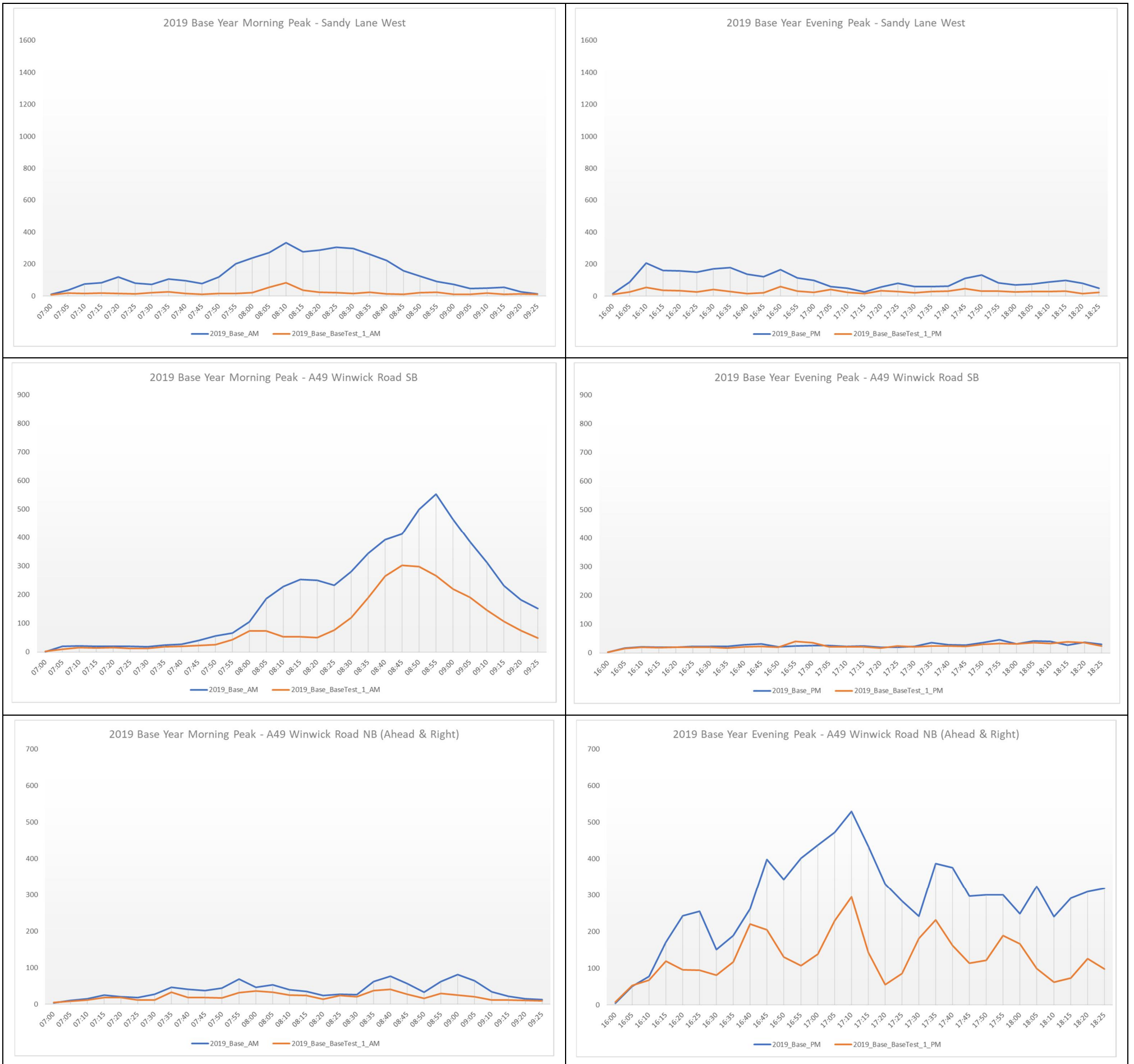
Figure GR3.18: 2019 Base Year Predicted VISSIM Model Queue Lengths at A49/Cromwell Avenue/Sandy Lane West Roundabout
