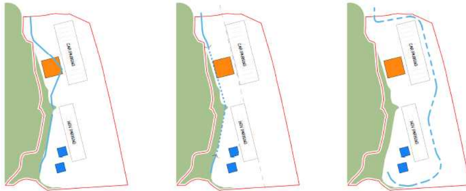
Figure 4.8: Brook diversion Options – Existing Location; Culverted; Diverted
