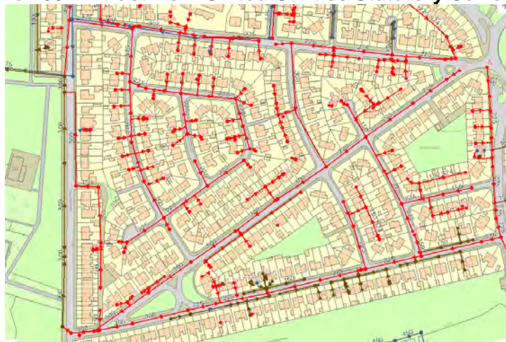
Figure 189: Extract from United Utilities Statutory Sewer Map
