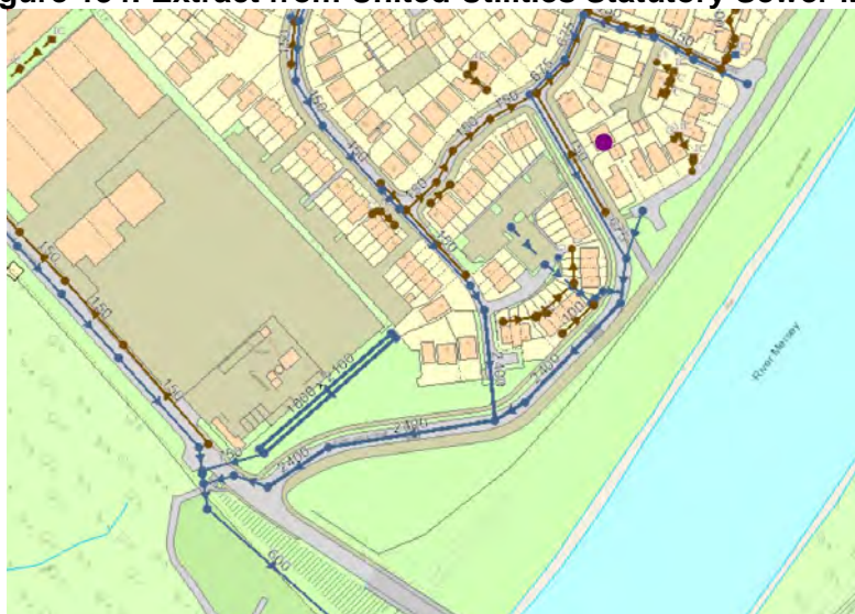
Figure 134: Extract from United Utilities Statutory Sewer Map
