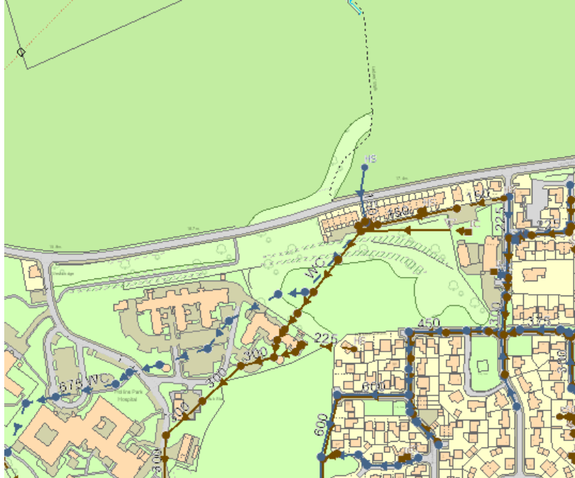
Figure 223: Extract from United Utilities Statutory Sewer Map
