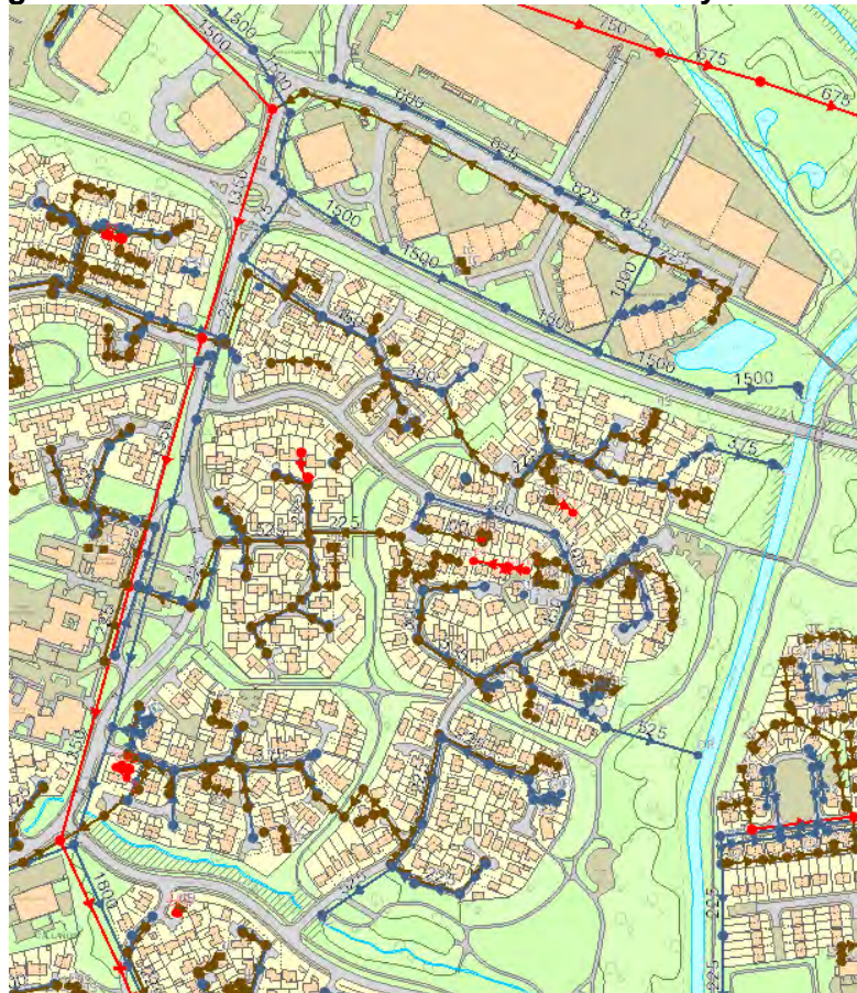
Figure 74: Extract from United Utilities Statutory Sewer Map
