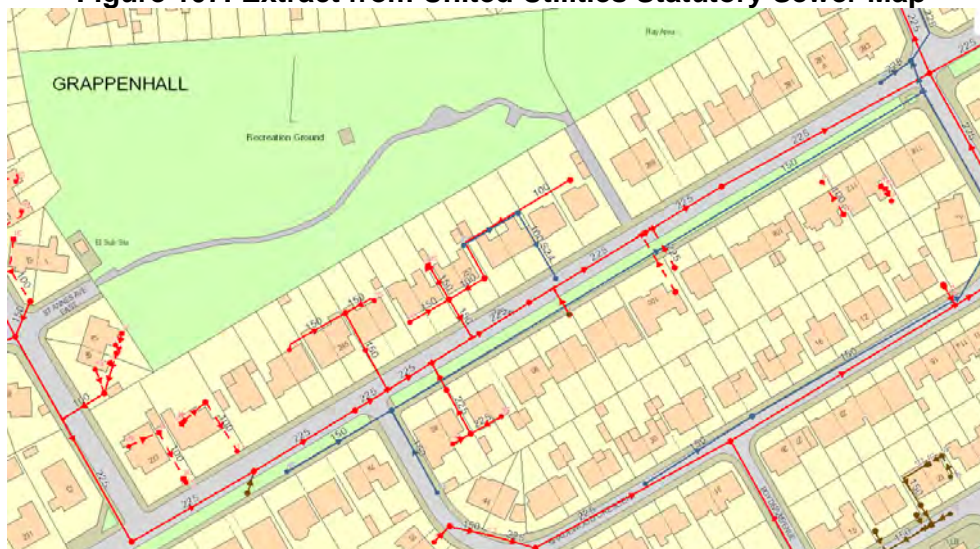
Figure 107: Extract from United Utilities Statutory Sewer Map
