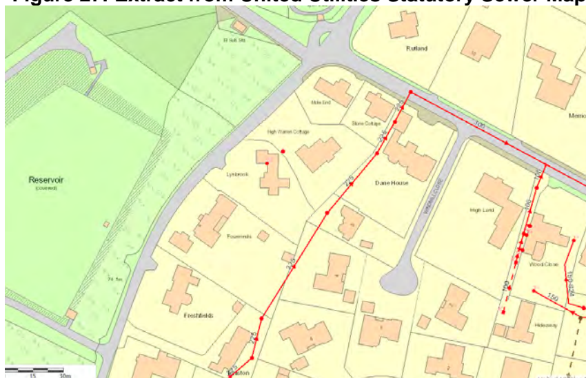
Figure 27: Extract from United Utilities Statutory Sewer Map
