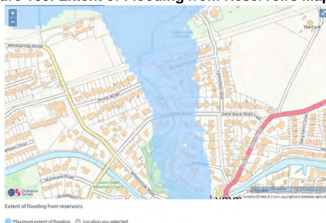
Figure 160: Extent of Flooding from Reservoirs Mapping
