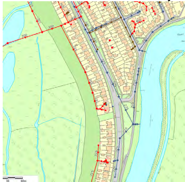
Figure 94: Extract from United Utilities Statutory Sewer Map
