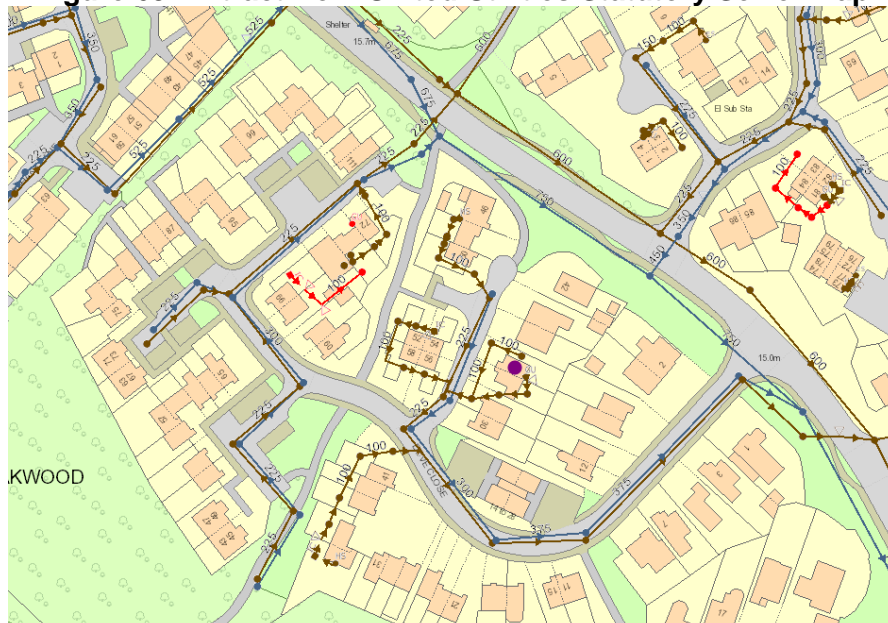
Figure 69: Extract from United Utilities Statutory Sewer Map
