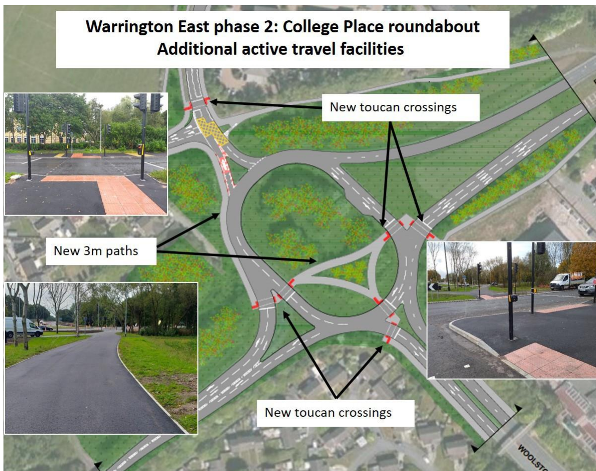
College Place roundabout – new crossings and paths
