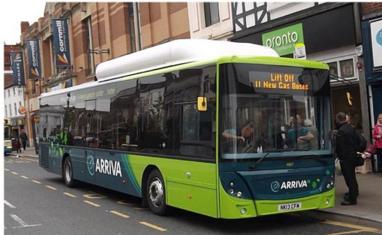
Figure 123 Arriva Hydrogen fuel cell bus - 70 passenger capacity
